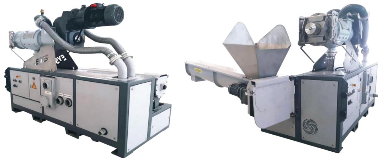
Separated solids can easily be transferred by a special conveyor which can be opened in seconds. Conveyor can be opened or closed by hand and locked by hinges easily. SEP2GO™ comes with a hand pump to adjust working position of discharge conveyor.
